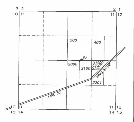
WELL#3 (LAKE 1386) PROPOSED & LOCATED IN THE SW 1/4 NE 1/4 SECTION 11, T28S R16E, W.M. LOCATED 30 FEET NORTH AND 780 FEET EAST FROM THE CENTER 1/4 CORNER OF SECTION 11.
