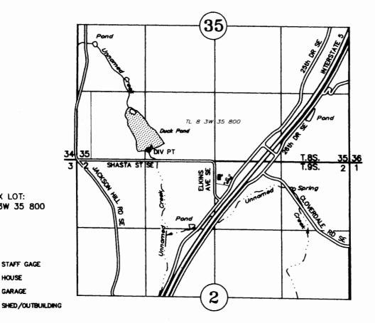
DIV PT: 190' NORTH AND 1385' EAST OF SW CORNER OF SECTION 35 STAFF GAGE: 240' NORTH AND 1435' EAST OF SW CORNER OF SECTION 35
