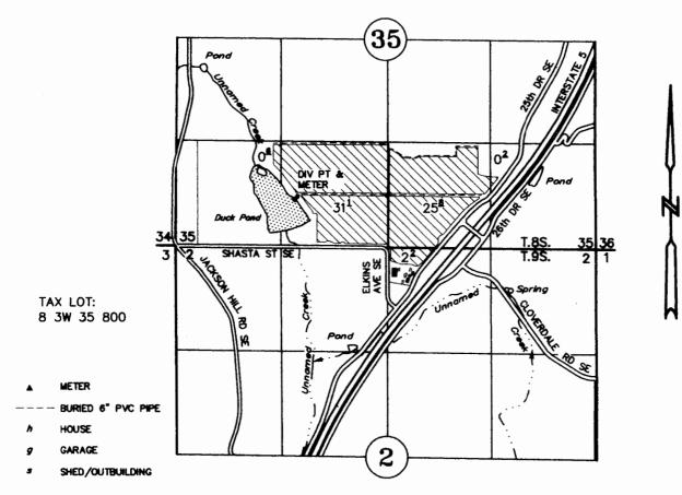
DIV PT: 570' NORTH AND 1505' EAST OF SW CORNER OF SECTION 35 METER: 585' NORTH AND 1520' EAST OF SW CORNER OF SECTION 35
