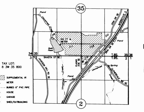
DIV PT: 570' NORTH AND 1505' EAST OF SW CORNER OF SECTION 35 METER: 585' NORTH AND 1520' EAST OF SW CORNER OF SECTION 35
