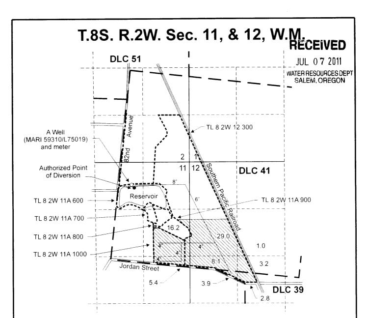
Authorized point of diverson (primary irrigation) is located 690 feet S. and 1,070 feet E. from the N 1/4 corner of Section 11. Authorized point of appropriation (MARI 59310/L75019, supplemental irrigation) is located 650 feet S. and 1,040 feet E. from the N 1/4 corner of Section 11.
