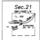
Authorized Div. Pt. 1 is 230' N. and 10' E. of the S1/4 Cor. Sec. 20-T-6167 Authorized Div. Pt. 2 (Oliver Ditch N. side) is 950' N. and 500' E. of the SW Cor. Sec. 21-T-6710 Authorized Div. Pt. 3 (Oliver Ditch S. side) is 900 N. and 1950' W of the SE Cor Sec. 21-S.0., V.13, P.95 Authorized Div. Pt. 4 is in the NE1/4NE1/4 Sec. 30-Per Adjudication Map -C-64330 Additional Div. Pt. is 330' N. and 25' W. of the S1/4 Cor. Sec. 20-T-6167
