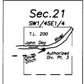
Authorized Div. Pt. 1 is 230' N. and 10' E. of the S1/4 Cor. Sec. 20-T-6167 Authorized Div. Pt. 2 (Oliver Ditch N. side) is 950' N. and 500' E. of the SW Cor. Sec. 21-T-6710 Authorized Div. Pt. 3 (Oliver Ditch S. side) is 900 N. and 1950' W of the SE Cor Sec. 21-S.O., V.13, P.95 Authorized Div. Pt. 4 is in the NE1/4NE1/4 Sec. 30-Per Adjudication Map -C-64330 Additional Div. Pt. is 330' N. and 25' W. of the S1/4 Cor. Sec. 20-T-6167
