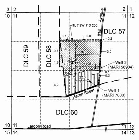
Weil 1 (MARI 7000) is located 720 feet north and 1,000 feet east from the SW corner of DLC 57. Well 2 (MARI 58904 is located 1,240 feet north and 1,450 feet east from the SW corner of DLC 57.
