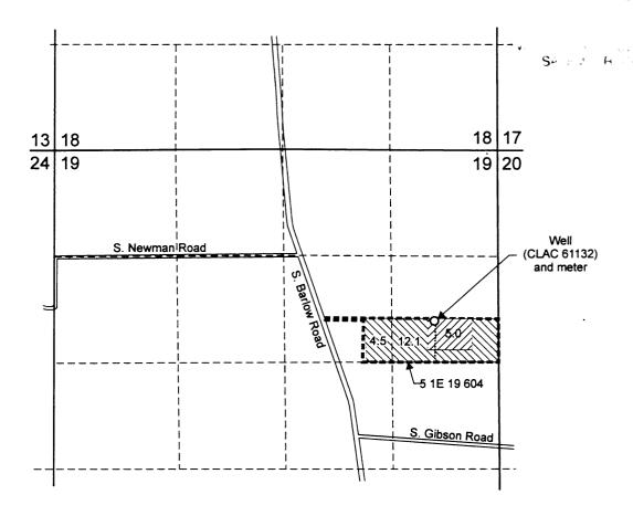
Well (CLAC 61132) is located 2,120 feet south and 770 feet west from the NE corner of Section 19.
