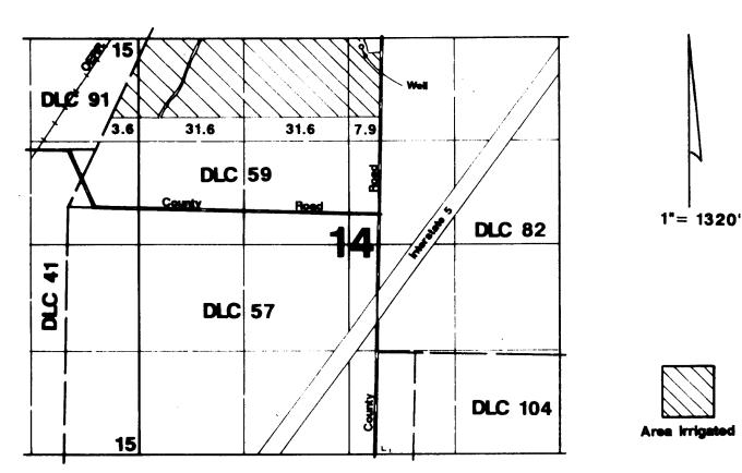
Well located 100'S & 2786'E from NW corner of Section 14.
