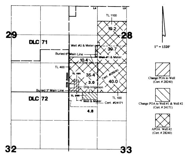
Well is located 387'S & 615'E from the SE corner of Section 29. Well #1 is located 1650'N & 1250'E from the SW corner of Section 28. Well #2 is located 2157'N & 1245'E from the SW corner of Section 28.
