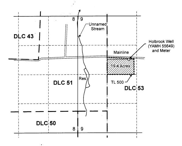
Holbrook Well (YAMH 55649) is located 3,335 feet north and 2,285 feet east from the SW corner of Section 9.
