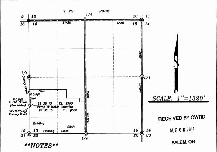
Pump Site with flowmeter is located 1260' South and 85' East of the West 1/4 corner of Section 15.
