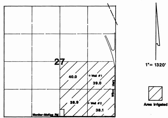
Well #1 located 1960'N & 1230'W from SE corner Section 27. Well #2 located 660'N & 1280'W from SE corner Section 27.
