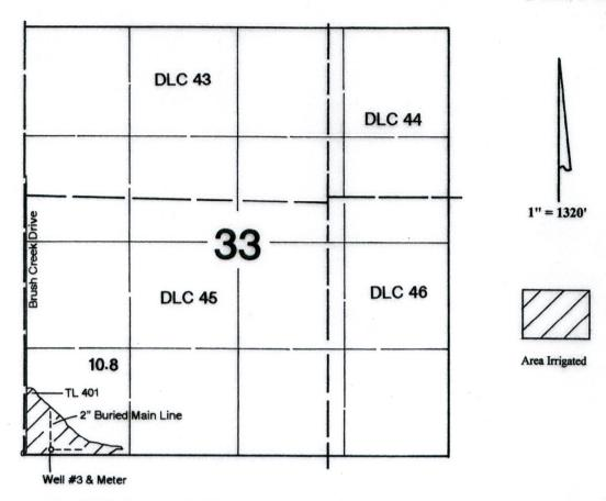
Well #3 is located 15' N & 355' E from the SW corner of Section 33.
