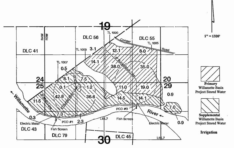
POD #1 is located S 580 15' W 42.5 chains from N1/4 corner Section 30. POD #3 is located S 58° 0' E 25.5 chains from N1/4 corner Section 30.
