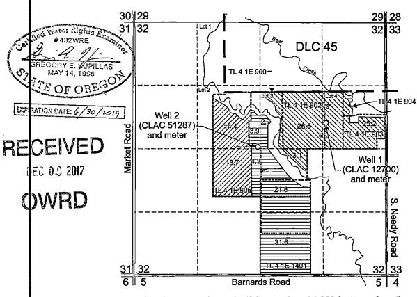
Well 1 (CLAC 12700) and meter are located 550 feet north and 1,250 feet west from the east 1/4 corner, Section 32.
