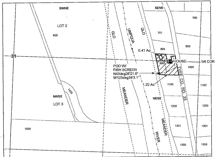
THE POD IS LOCATED AT 603 FEET WEST AND 183 FEET SOUTH OF THE EAST 1/4 CORNER OF SECTION 31
