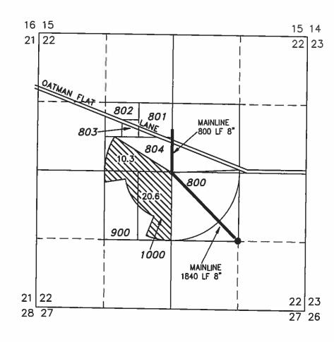
POA LAKE 733 IS LOCATED IN THE NW 1/4 SE 1/4 SECTION 22, T27S R13E, W.M. LOCATED 10 FEET NORTH AND 1310 FEET EAST FROM THE CENTER—SOUTH SIXTEENTH CORNER OF SECTION 22.
