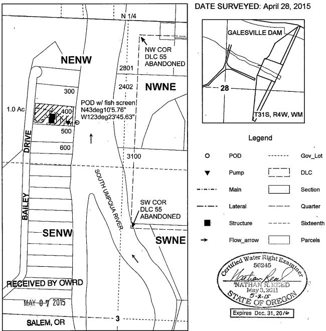
POD IS LOCATED 410 FEET WEST AND 910 FEET SOUTH OF THE N1/4 OF SECTION 3.
