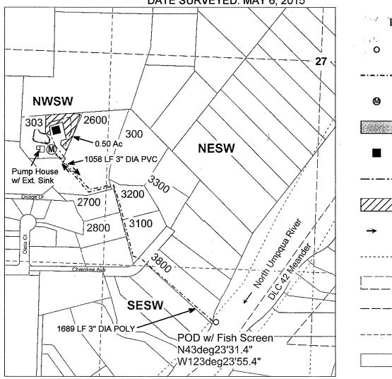
POD IS LOCATED1640 FEET SOUTH AND 635 FEET WEST FROM THE CENTER OF SECTION 27.
