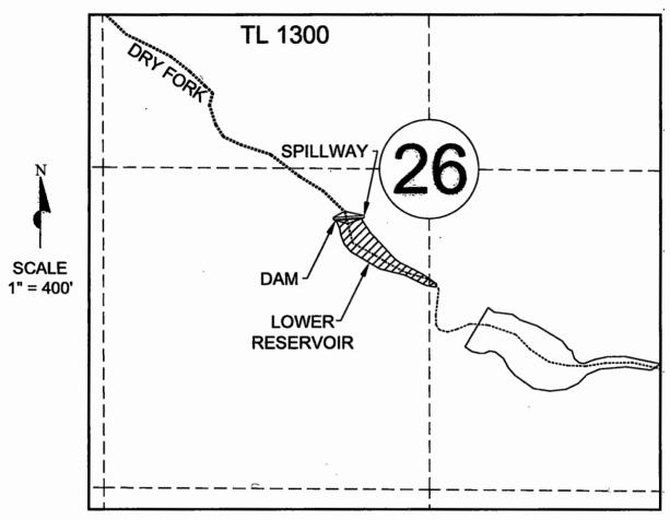
CENTER OF DAM LOCATED 200 FEET SOUTH & 320 FEET WEST FROM THE CENTER OF SECTION 26
