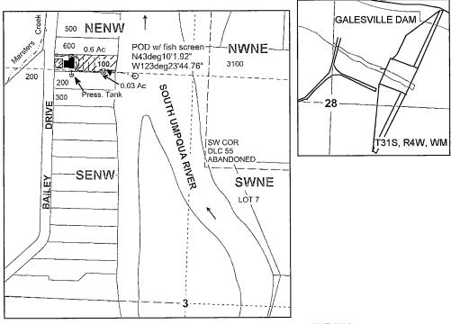
POD IS LOCATED 305 FEET WEST AND 1338 FEET NORTH OF THE C1/4 OF SECTION 3.
