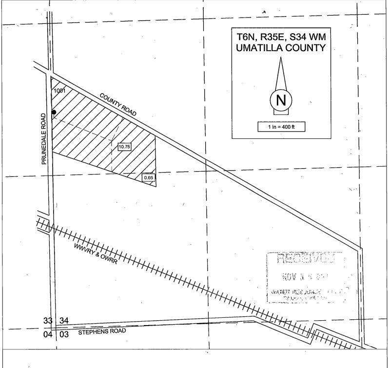
POA is basalt groundwater well located in the NW/4, SW/4, Section 34, T6N, R35E, WM, 776 feet South and 20 feet East from the W 1/4 Corner of Section 34. Flow Meter is located at same location.
