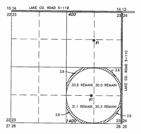
● WELL#3 (LAKE 52251) LOCATED IN THE NW 1/4 SE 1/4 SECTION 23, T25S R14E, W.M. LOCATED 1320 FEET SOUTH AND 1450 FEET WEST FROM THE EAST 1/4 CORNER OF SECTION 23.
