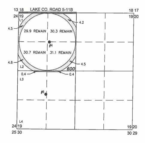
WELL#4 (LAKE 171) LOCATED IN THE NE 1/4 NW 1/4 SECTION 19, T25S R15E, W.M. LOCATED 1330 FEET SOUTH AND 1440 FEET EAST FROM THE NORTHWEST CORNER OF SECTION 19.
