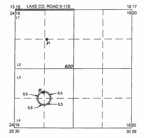
• WELL#6 (LAKE 170/174) LOCATED IN THE NW 1/4 SW 1/4 SECTION 19, T25S R15E, W.M. LOCATED 3700 FEET SOUTH AND 1310 FEET EAST FROM THE NW CORNER OF SECTION 19.
