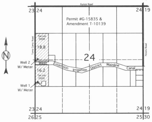
Well 1 Located 1260' S & 311' E of W 1/4 Corner Section 24, NW1/4 of SW1/4 (Lat. N 45° 48' 39.23076", Lon. W 119° 46' 11.08507") W/ Meter Well 2 Located 28' N & 172' E of W 1/4 Corner Section 24, SW1/4 of NW1/4 (Lat. N 45°48' 49.06969", Lon. W 119° 46' 09.92576") W/ Meter
