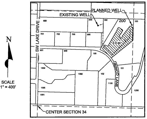
EXISTING WELL: LOCATED 1120' NORTH AND 820' EAST FROM CENTER OF SECTION 34 (1530' SOUTH AND 1810' WEST FROM NE CORNER OF SECTION 34)
