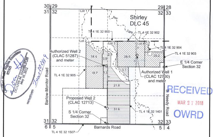
Authorized Well 1 (CLAC 12700) and meter are located 550 feet north and 1,250 feet west from the east 1/4 corner, Section 32.
