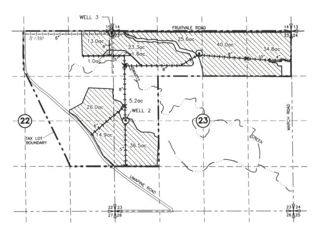
POINTS OF APPROPRIATION WELL NO 2 LOCATED 2660' NORTH AND 350' EAST FROM THE SW CORNER SECTION 23 METER LOCATED AT WELL SITE
