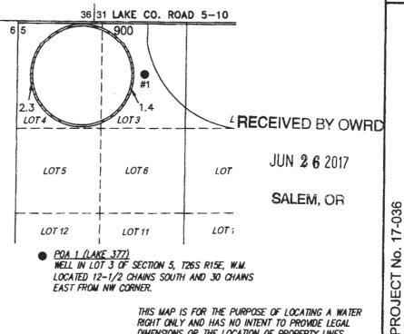
POA 1 (LAKE 377) WELL IN LOT 3 OF SECTION 5, T26S R15E, W.M. LOCATED 12-1/2 CHAINS SOUTH AND 30 CHAINS EAST FROM NW CORNER.
