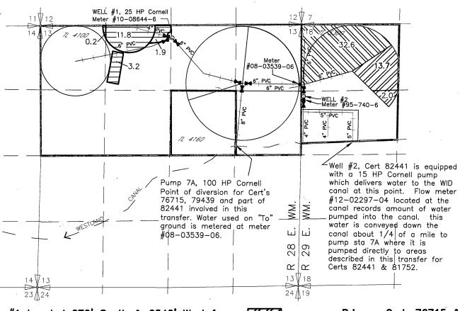
WELL #1 Located 270' South & 2540' West from the NE corner section 13, T3N, R28E, WM WELL #2 Located 1450' South & 3160' West from the N 1/4 corner section 18, T3N, R29E, WM T3N., R 29E., W.M.
