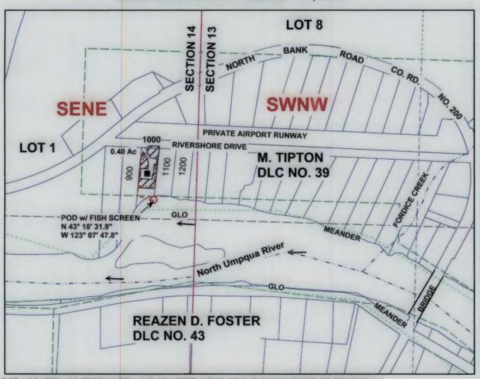
POD LOCATED 108 FEET NORTH AND 251 FEET WEST OF THE E1/4 CORNER OF SECTION 14
