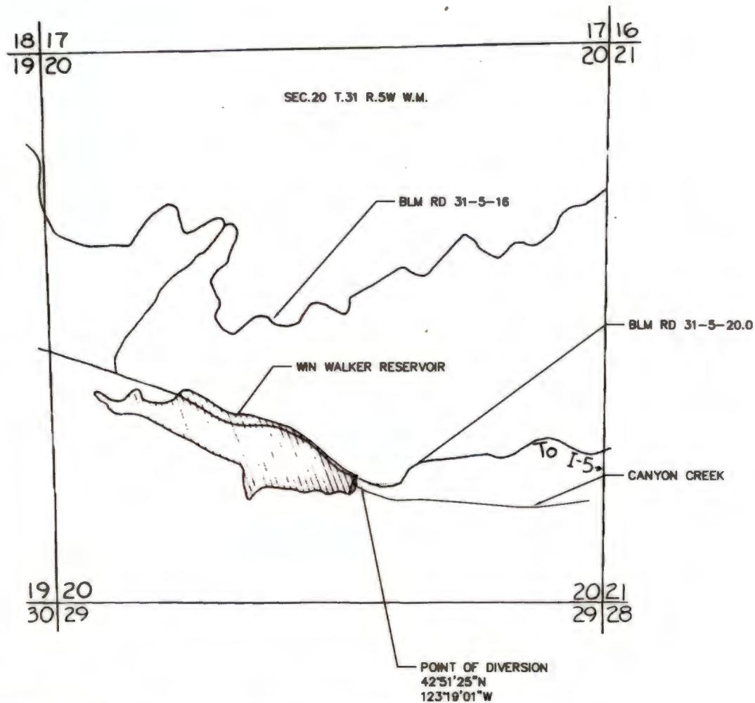
THE POINT OF DIVERSION IS LOCATED 1,114 FEET NORTH AND 2,532 FEET WEST FROM THE SOUTHEAST CORNER OF SECTION 20, BEING WITHIN THE SW 1/4 SE 1/4 OF SECTION 20, TOWNSHIP 31 SOUTH, RANGE 5 WEST, W.M. IN THE COUNTY OF DOUGLAS.
