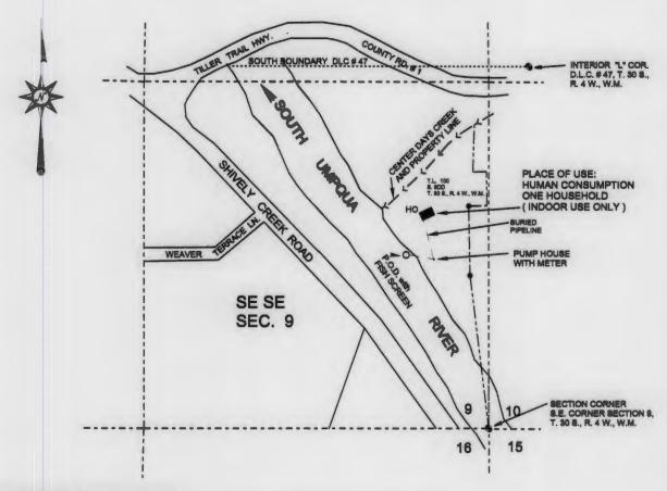
POD IS 661 FEET NORTH AND 316 FEET WEST OF THE SOUTHEAST SECTION CORNER OF SECTION 9, TOWNSHIP 30 SOUTH, RANGE 4 WEST, WILLAMETTE MERIDIAN. METER BEARS SOUTH 81\* 39' 36" EAST 107 FEET FROM POD.
