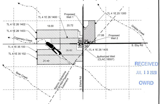
Authorized Well (CLAC 18557) is located 15 feet north and 280 feet west from the SE corner, Section 26. Proposed Well 1 is located 875 feet north and 105 feet east from the SW corner, Section 25. Proposed Well 2 is located 65 feet north and 185 feet east from the SW corner, Section 25.
