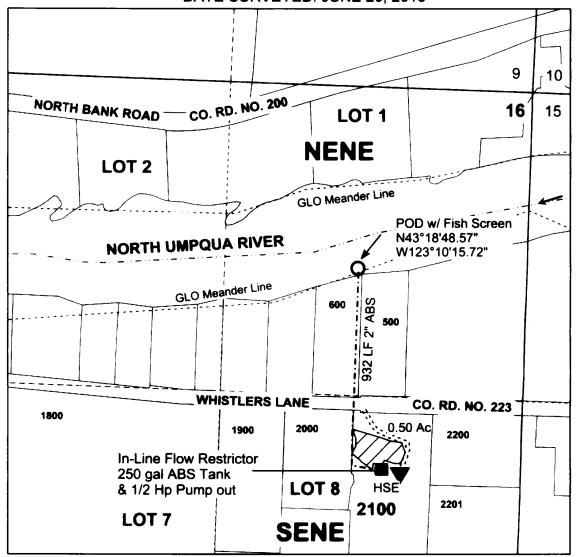
POD IS LOCATED 775 FEET SOUTH AND 765 FEET WEST FROM THE NORTHEAST CORNER OF SECTION 16  $\,$
