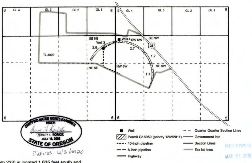
Well 3 (Malh 223) is located 1,635 feet south and 555 feet west of the NE corner of section 6.
