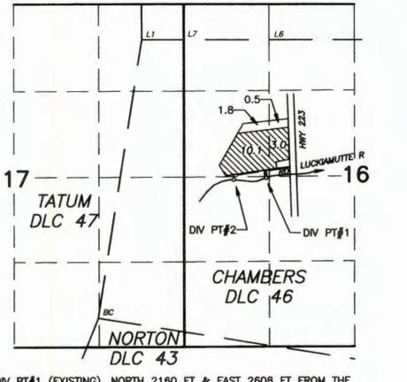
DIV PT#1 (EXISTING), NORTH 2160 FT & EAST 2608 FT FROM THE SW CORNER, CHAMBERS DLC #46 DIV PT #2 (NEW) NORTH 2680 FT AND EAST 2910 FEET FROM THE SW CORNER, CHAMBERS DLC #46
