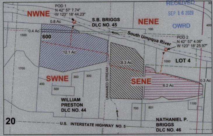
POD 1 IS LOCATED 1517 FEET NORTH AND 846 FEET EAST FROM THE C1/4 CORNER OF SECTION 20 AS PROJECTED WITHIN DLC NO. 45.
