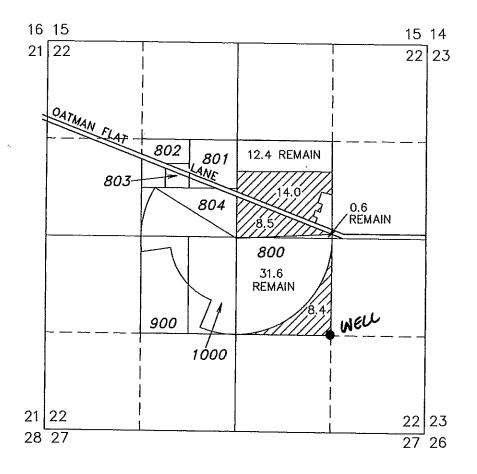
POA LAKE 733 IS LOCATED IN THE NW 1/4 SE 1/4 SECTION 22, T27S R13E, W.M. LOCATED 10 FEET NORTH AND 1310 FEET EAST FROM THE CENTER—SOUTH SIXTEENTH CORNER OF SECTION 22.
