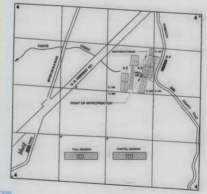
THE POINT OF APPROPRIATION IS LOCATED 1745 FEET SOUTH AND 1690 FEET WEST FROM THE NORTHEAST CORNER OF SECTION 4; BEING WITHIN THE SW'/NE'/LOF SECTION 4, TOWNSHIP 28 SOUTH, RANGE 14 WEST, W.M., COOS COUNTY.
