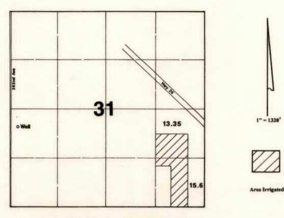
Well is located 450'S & 216'E from the W1/4 corner of Section 31.
