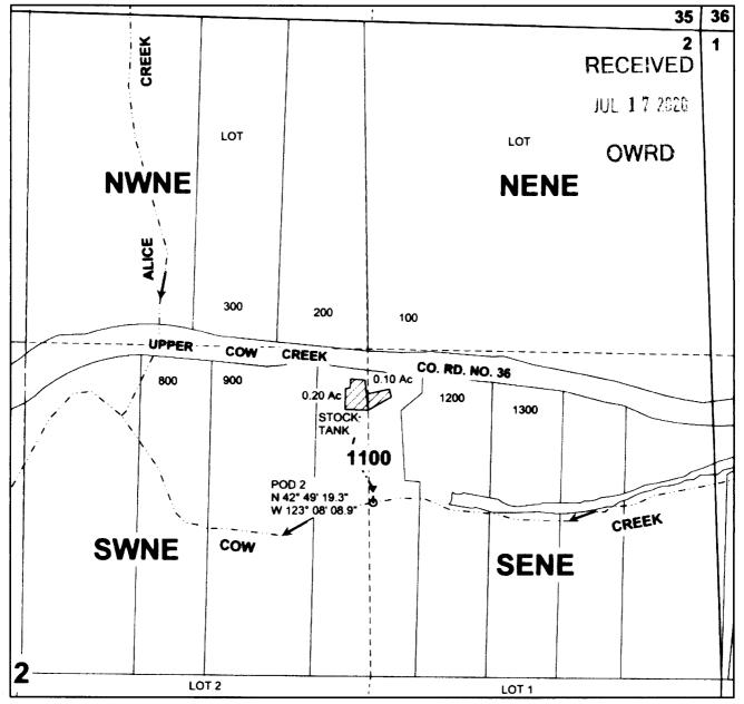
POD 2 IS LOCATED 689 FEET NORTH AND 1340 FEET EAST OF C1/4 OF SECTION 2.
