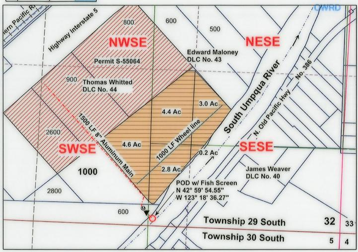
POD IS LOCATED 63 FEET NORTH AND 1024 FEET WEST FROM THE SE CORNER OF SECTION 32 East 51/4 Legend MAP PREPARED FOR: CITY of MYRTLE CREEK POD DLC **PO BOX 940** Stream MYRTLE CREEK, OR 97457 Wiled Water Right Ex **PUMP Pipeline** Quarter Meter Flow arrow Sixteenth
