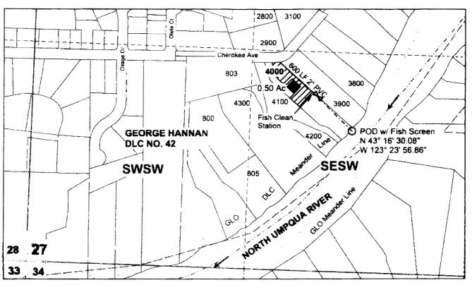
POD IS LOCATED 810 FEET NORTH AND 1960 FEET EAST FROM THE SW CORNER, SECTION 27 AS PROJECTED IN DLC NO. 42.
