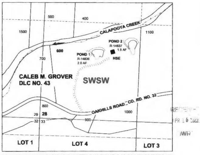
POND 1 IS LOCATED 915 FEET NORTH AND 750 FEET EAST FROM THE SW CORNER OF SECTION 28 AS PROJECTED WITHIN DLC NO. 43.
