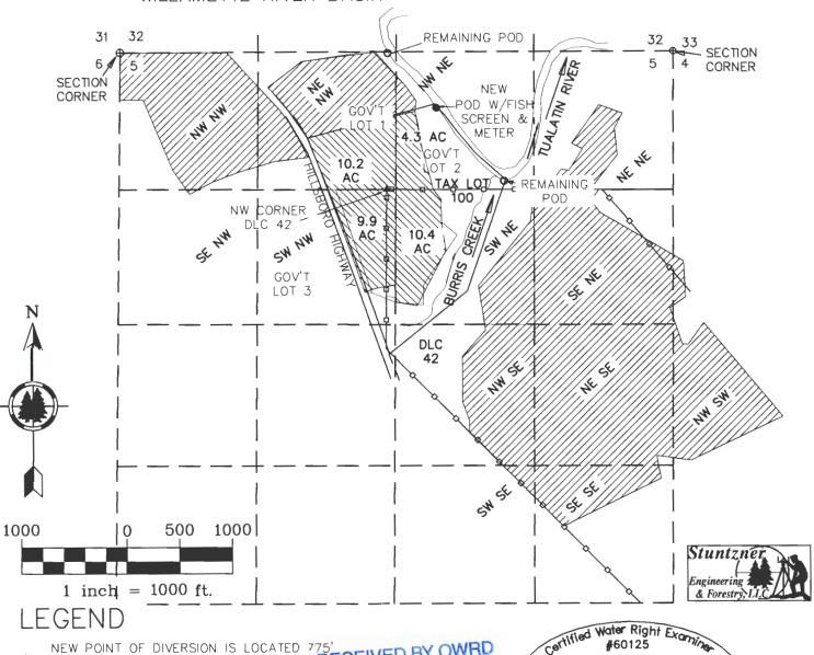
NEW POINT OF DIVERSION IS LOCATED 775' NORTH AND 440' EAST OF THE NW COR. POFCEIVED BY OWRD DLC 42 WITH METER AND FISH SCREEN
