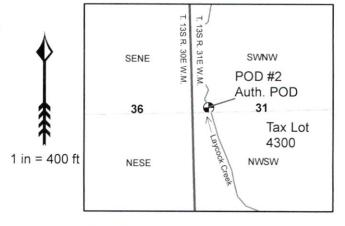
Auth POD located approximately: 90 ft. S, 89 ft E from the east 1/4 Corner of Section 36, T. 13S R. 30 E W.M. As established by Transfer B-105
