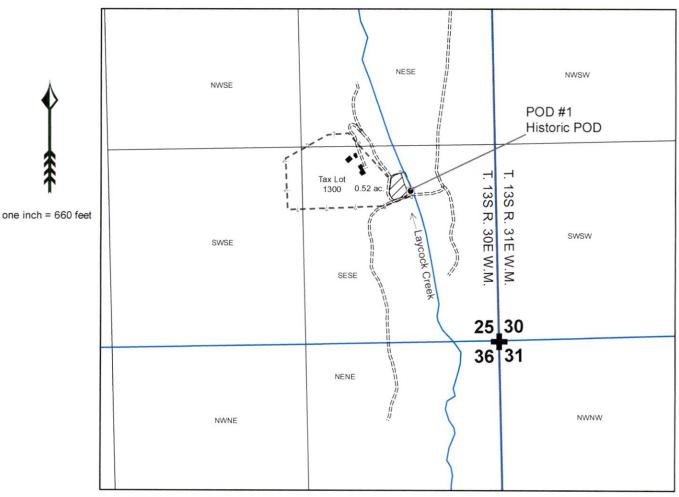
POD #1 Historic Point of Diversion is located approximately: 1024 ft. N and 584 ft. W of the NE Corner of Section 36, T. 13S R. 30E. W.M.
